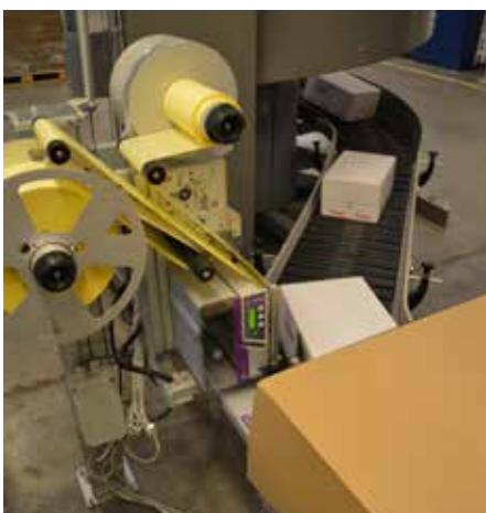
Label applicators receive all necessary product data from the M3 business system via CodeIT Enterprise. Shown here are labelled distribution packages for popular Norwegian Soppas Pasta.
